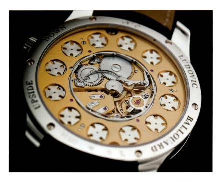
The clear caseback reveals the 12 Maltese crosses used to rotate the individual hour discs along with the movement, which is crafted from brass giving it a distinctive radiance.
